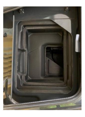
Create manifold to size of fresh air intake housing. Install Flange Kit onto the manifold.
